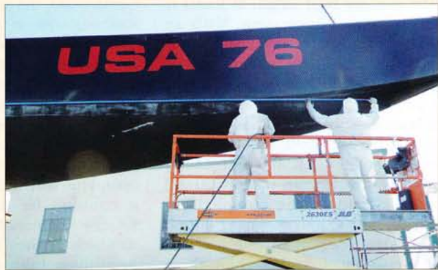
Crews tape the waterline of USA 76 in KKMI's Point Richmond yard. In 2011 the yard converted the 2001 America's Cup boat for day-charter service.
