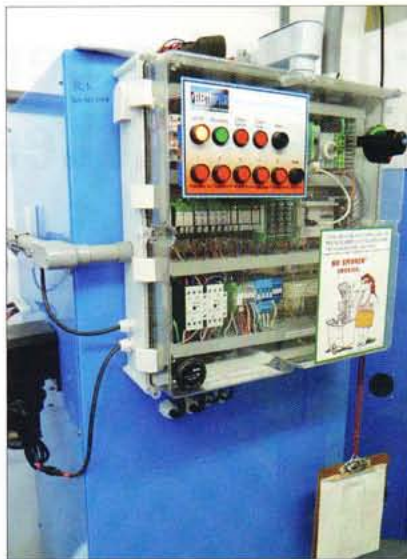
The ElectroPulse system from OilTrap Environmental (Tumwater, Washington) is wired to a central control panel (left). It adjusts the pH of the wastewater before sending it through a series of 4"-diameter (102mm) tubes fitted with electrically charged plates (right) that change the polarity of any suspended solids, causing them to cluster and float, and rendering any metals inert through oxidization.
