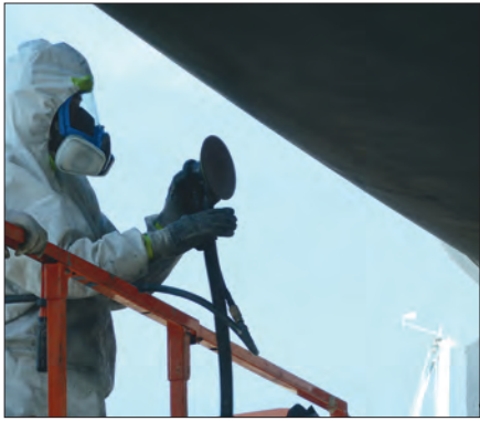
Above —Years of experience has led KKMI to conclude that for sanding, vacuum sanders and tarping are a better solution to trap particles and meet air emission standards than wet-sanding, which requires disposal of an even larger mess of contaminated water. Right —An open-topped shipping container covered in clear plastic serves as a reasonably priced spray booth with good ambient light and no risk of explosion from electric lights.
