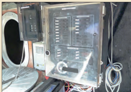
Changes to USA 76 included, from left to right: an electrical system complete with panel; a Yanmar auxiliary engine with attendant fuel tank, fire-suppression systems, and ventilation; and five watertight bulkheads, one shown here with a watertight penetration open.
