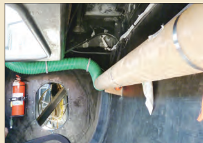
Changes to USA 76 included, from left to right: an electrical system complete with panel; a Yanmar auxiliary engine with attendant fuel tank, fire-suppression systems, and ventilation; and five watertight bulkheads, one shown here with a watertight penetration open.
