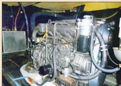
Changes to USA 76 included, from left to right: an electrical system complete with panel; a Yanmar auxiliary engine with attendant fuel tank, fire-suppression systems, and ventilation; and five watertight bulkheads, one shown here with a watertight penetration open.
